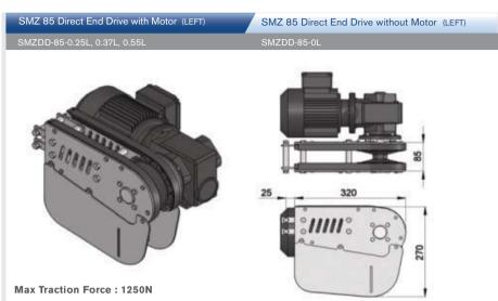
The Direct End Drive Unit is without torque limiter. Standard attached gear motors are with SEW motor size 0.25kW, 0.37kW & 0.55kW. SMZDD-85-0L represents direct drive without motor. Multi channel drives available upon request.
